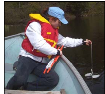
A Lake Partner Program volunteer uses a Secchi disk to measure water clarity in a lake.
