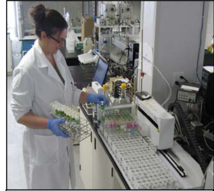
Chemistry Technician at the Dorset Environmental Science Centre performs total phosphorus analyses on Lake Partner Program water samples.
